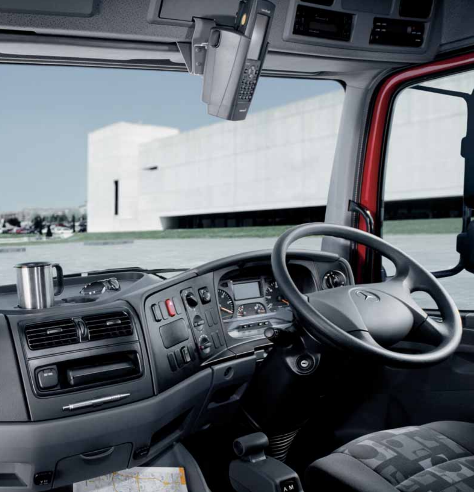
In the "Long-distance" cockpit, the extended instrument panel provides further generously sized stowage options. The brake lever is integrated in the instrument panel.
