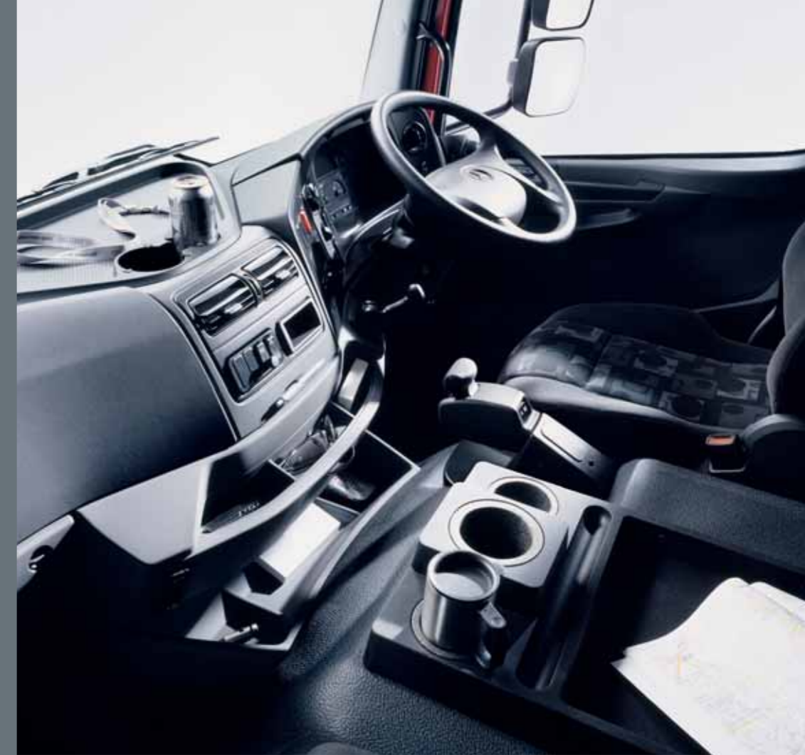
In the "Long-distance" cockpit, the extended instrument panel provides further generously sized stowage options. The brake lever is integrated in the instrument panel.
