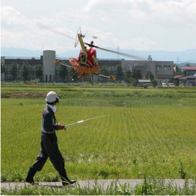
Radio Controlled (RC) helicopter used to spray crops. Along the road in northern Japan. Photo by Stephanie Hackney.
