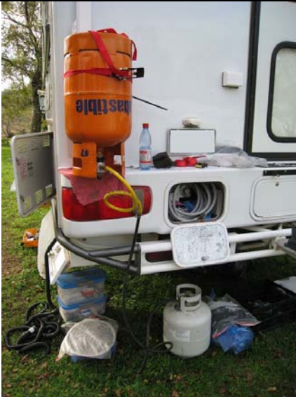
Jumper test of Chilean 11kg bottle. Note feeder tank securely attached to elevated position with ratchet strap. Note feeder bottle in sun, target tank in shade.
