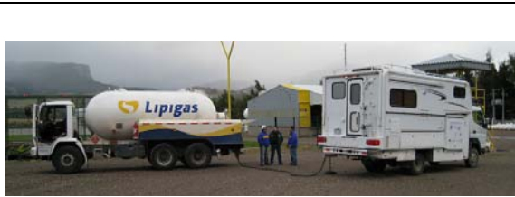
Refilling from a bobtail delivery truck. Coihaique, Chile.
