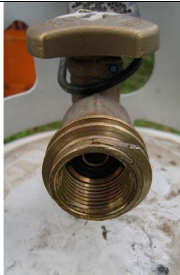
QCC Type 1 connector with POL threads on the interior of the hose connection.
