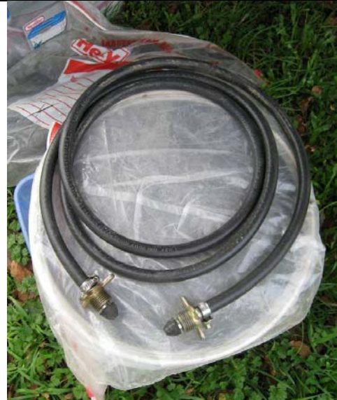
POL to POL hose used for jumper fill. Note this hose is rated for liquid propane.
