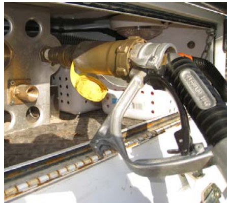
Vehicle propane/LPG refill pump connector
