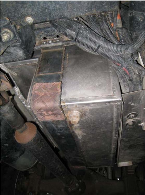
Forward end of the repaired and reinforced bracket.
