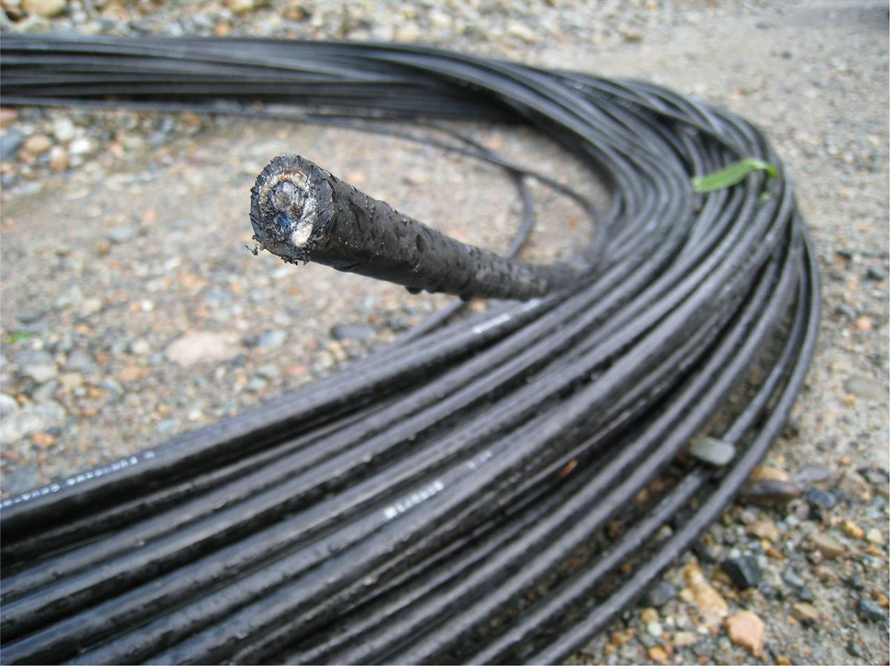
The coil of new optical fiber cable used to patch the cable broken by the flood.
