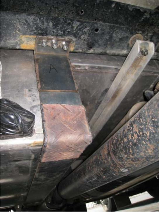
Aft end of the repaired and reinforced bracket.
