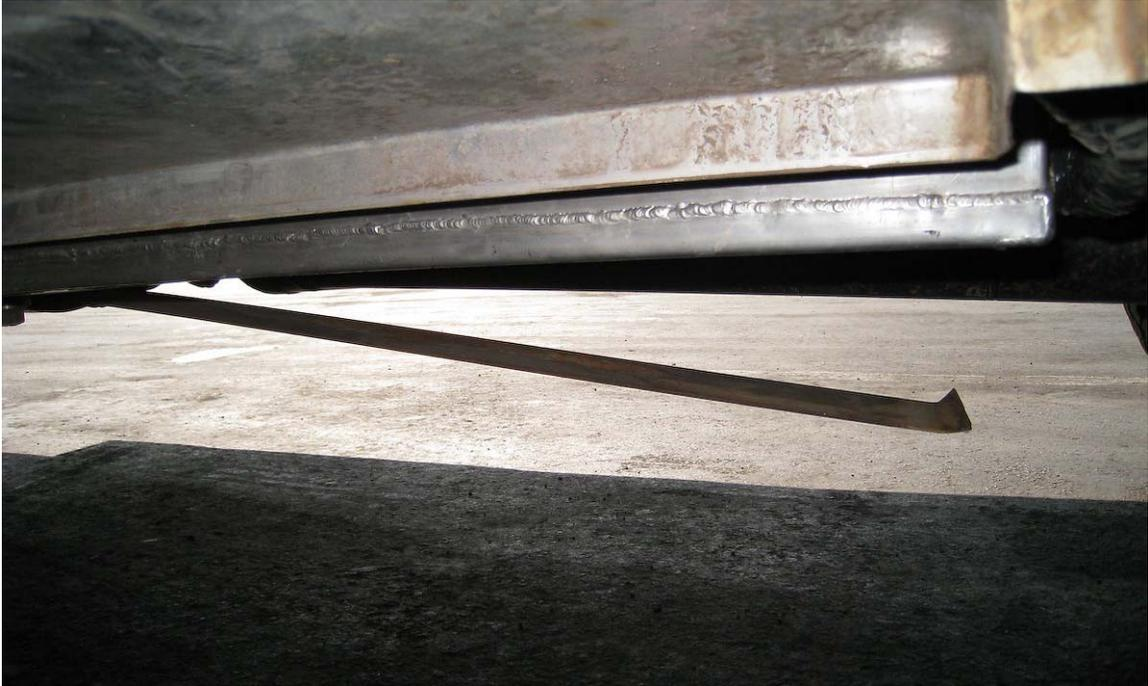
My initial view of the broken raw water tank bracket.
