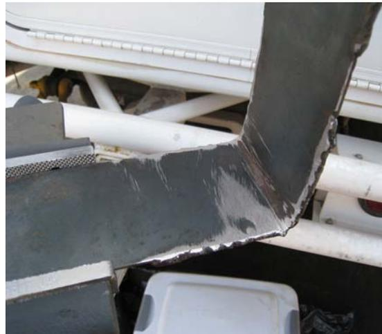
Smoothing off the welds so they wouldn't wear through the tank. I thought the vise would be dead weight and one of the first things we ejected to reduce weight. As it has turned out, I couldn't begin to count the number of times I've used it.
