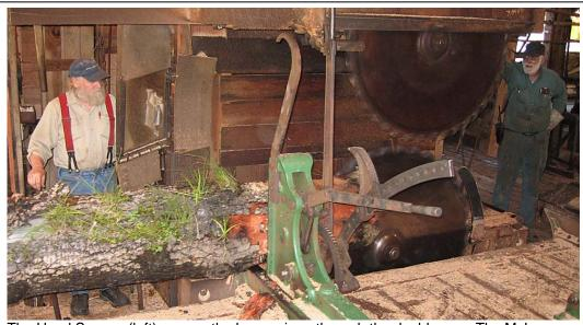
The Head Sawyer (left) passes the log carriage through the double saw. The McLean mill is now unique in its ability to cut lumber of long lengths and large dimension, as modern mills are designed to only cut common lumber lengths and dimensions.
