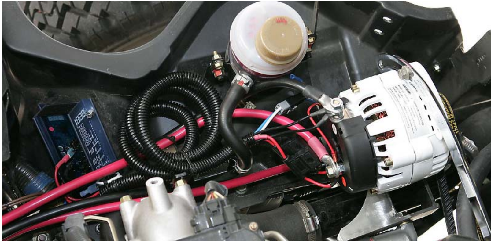
Dedicated Balmar alternator and 3 stage voltage regulator
