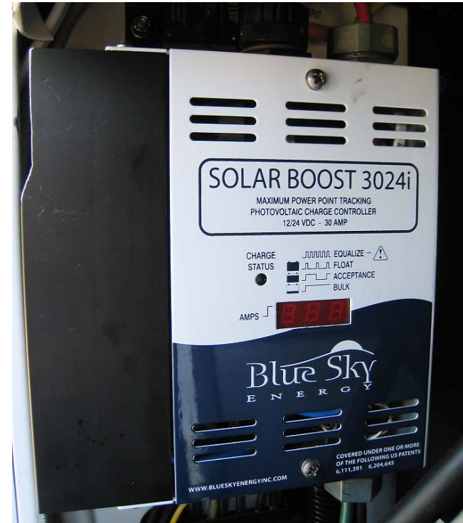
Solar controller / 3 stage charger
