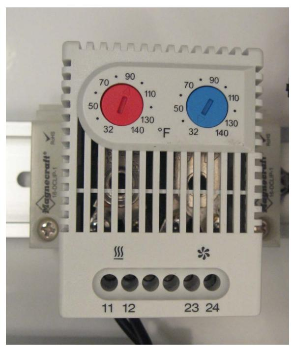
Starting with the thermostat, which doesn't really run on any voltage, it just latches closed a contact if the temp exceeds or drops below the relevant setting.
