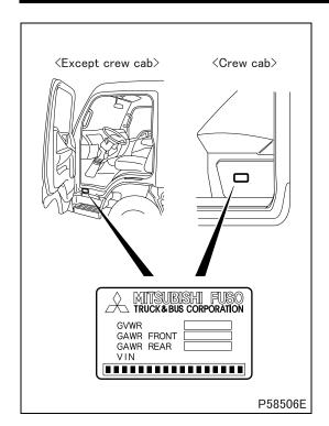
The vehicle identification number is punch-marked on the plate, which is attached in the position as illustrated.
