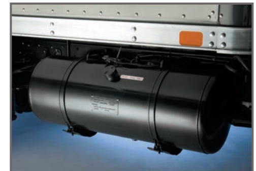
In-dash windshield fluid fill Covered, open-grate steps stay cleaner Standard 33-gallon side-mounted fuel tank
